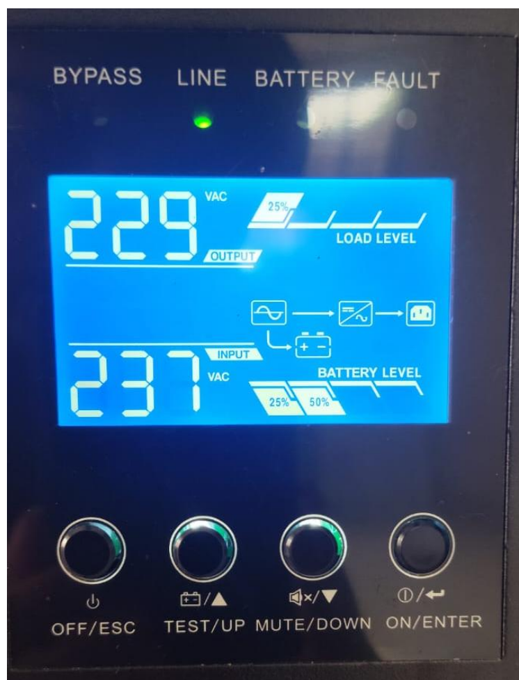
Figura 21, Panel de control del UPS Smarbit. 33
